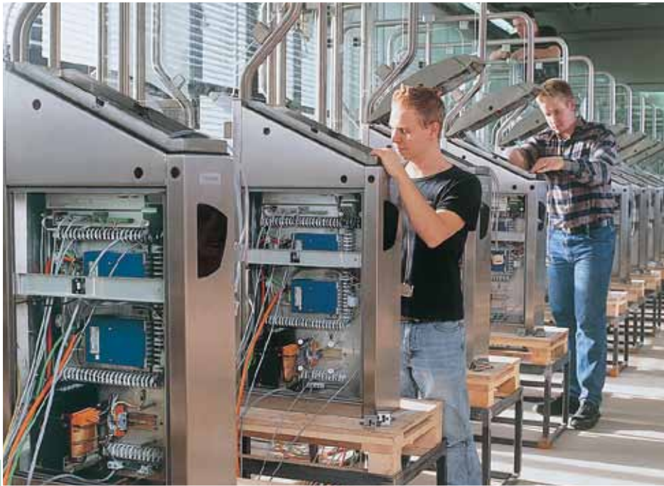
Above: Skilled specialists at Magnetic Autocontrol GmbH, Germany assembling fare collection access control gates for installation in the Netherlands.
